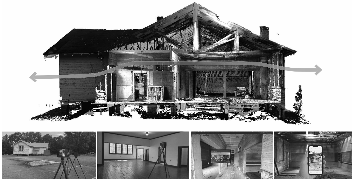
Figure 3. Point cloud of Tankersley Rosenwald School, showing the passive design strategies (top), and the digital documentation technology including LiDAR Scanners, Photogrammetry Cameras, Immersive Digital Environment, and iPhone 13 Pro equipped with LiDAR (bottom, respectively). (Images provided by author).
